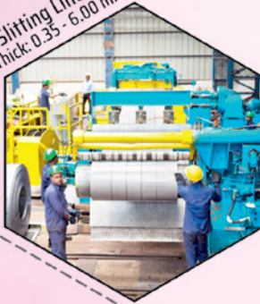
Slitting Line - 2 Thick: 0.35 - 2.50 mm
